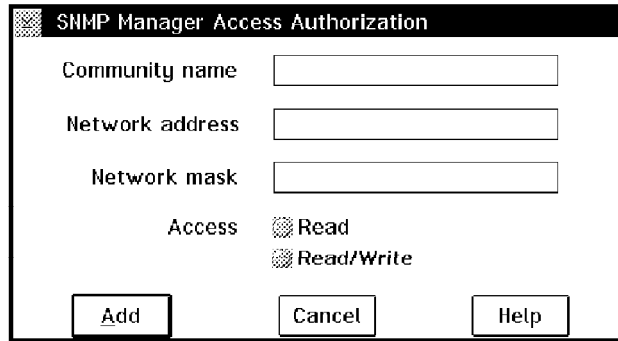
Figure 147. TCP/IP Services SNMP Page 2 - SNMP Manager Access Authorization
