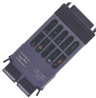
Figure 98. Short-wave GBIC (left) and a media interface adapter (MIA).
