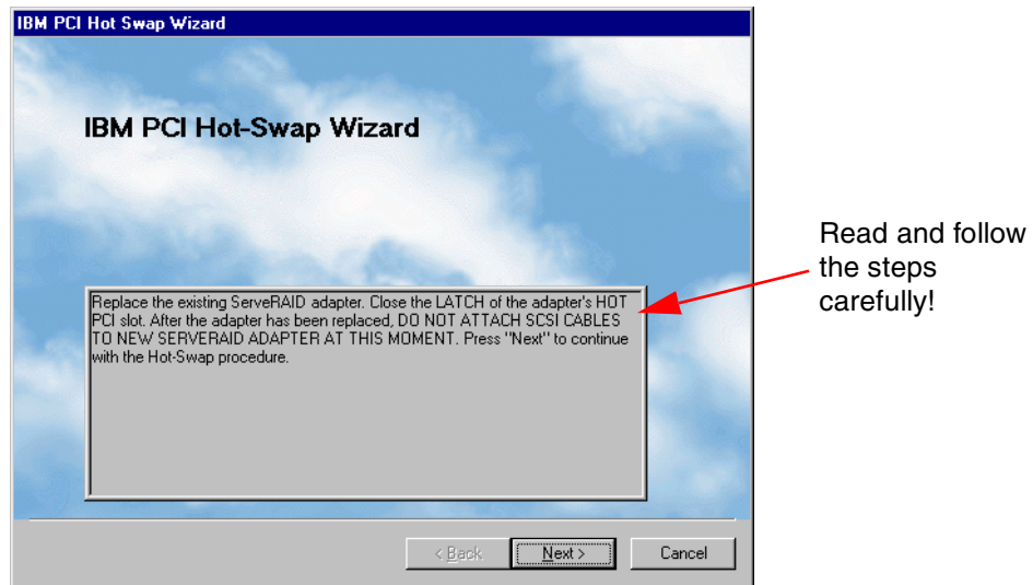
Figure 59. Hot-Swap Wizard - replacing a ServeRAID adapter
