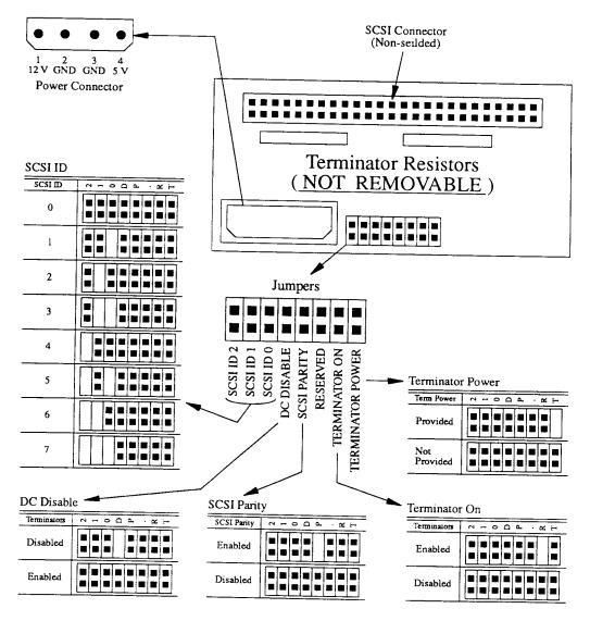
Note:  $\Box$  = CLOSED Jumper installed  $\blacksquare$  = OPEN Jumper not installed
