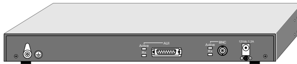
Rear Panel of the Model EN116 hub
