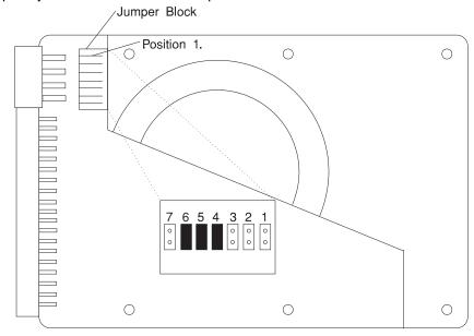
Refer to the above illustration, then locate positions 5, 6, and 7 on your drive. These positions are always used to set the SCSI address on the 1080MB SCSI-2 Disk Drive. In this example, jumpers are installed in positions 5 and 6, which sets the SCSI address to 6.
