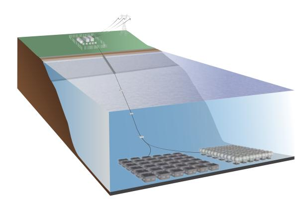
The air is then directed to an air cavity located 100+ meters below the surface of the water where the energy is stored at the same pressure as the water around it. The deeper the water is and closer to shore, the higher the pressures and more cost effective the storage solution becomes.
