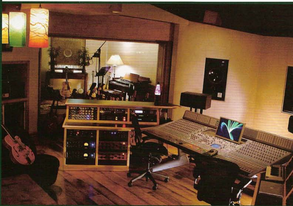
Control Room looking into Iso 1. Guitar amp rack on the far left. This features Marshall, Two-Rock, Ampeg, Fender, Vox, and Rockman amps that can be patched into cabinets in any room. Also contained is a Radial JD7 splitter, Demeter Spring Reverb, Korg Rack Tuner, and assorted guitar effects. This allows guitar and bass players to play in the control room with full control over the amps while the cabinet is blasting away in the other room. Digidesign ICON D – Control for Pro Tools HD4 Accel, Version 7.3.
