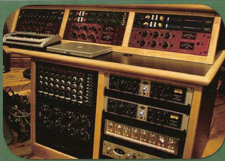
RIGHT CONSOLE RACK. Preamps are Great River MP2NV w/ EQ2NV, two Requisite Audio Pal Plus MkIII (Jamie's favourite!), two Chandler TG Channel's, two Chandler Germaniums, six Neve 1073s, two Neve 1084s, Shadow Hills GAMA 8, Grace 801, two UA 6176s, two Avalon US's, and a Requisite Audio L2M MkII Mastering Limiter. Mics in the other rooms can be hardwired to the preamps and then directly into the Mytek convertors, bypassing the patch bay. Jamie has custom Requisite audio cable for this purpose and although manual patching is required he says the quality gained is really stunning.
