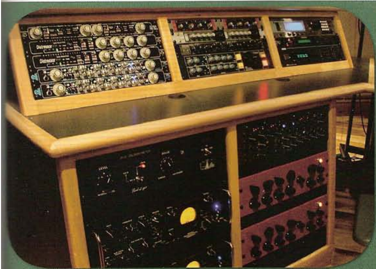
LEFT CONSOLE RACK. EQs and effect processors. Compressors are two Distressors and a Fatso Jr. by Empirical Labs, two tube Glory Comps, a pair of Neve Portico 5042 tape simulators, Smart Research C2 and a Neve 33609JD. EQs are two Empirical Labs Lil' Freq's, Dolby 740, Manley Massive Passive, and two DW Fearn VT4s. Effects are an Eventide H9000FW, Ensoniq DP Pro, and a Lexicon 300.
