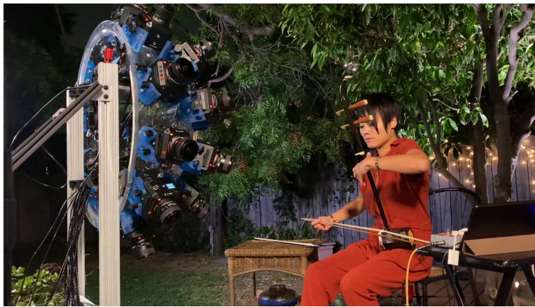
Figure 1: Our mid-range light field video camera array (left) consisting of 24 Z CAM E2 professional 4K cinema cameras mounted to a sturdy acrylic hemisphere is seen recording a performance of a traditional erhu instrument.
