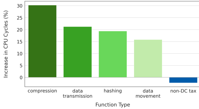
Figure 12. Aggregated change in CPU cycles (%) from Hard Limoncello. Data center tax functions (green) increased in CPU cycles under Hard Limoncello. In contrast, overall non-data center tax functions (blue) decreased in cycles.
