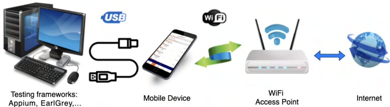
Fig. 4 - Typical mobile test architecture.
