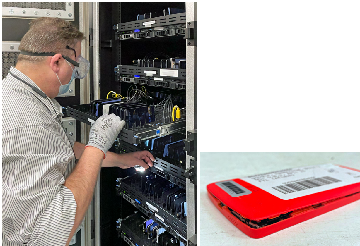
Fig. 17 - Visual inspection of the devices with swollen batteries, and a mobile device with swollen battery.
