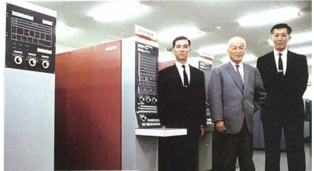
The FACOM 230-60, the first computer in the world to be made entirely with integrated circuits
