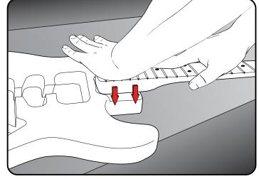
Press neck into neck pocket heel-first at a slight angle. Undue force should not be necessary.
