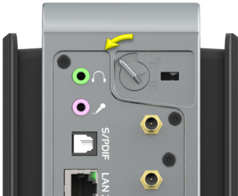
Figure 1 – Move locking knob to open position
