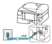
**Note:** If you're connecting to a DSL phone line, you must use a DSL filter or you won't be able to fax. Contact your DSL provider for the necessary filter.
