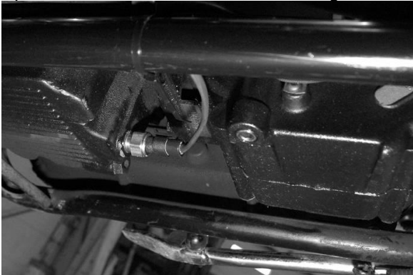
Installed oil temp sensor and harness plug
