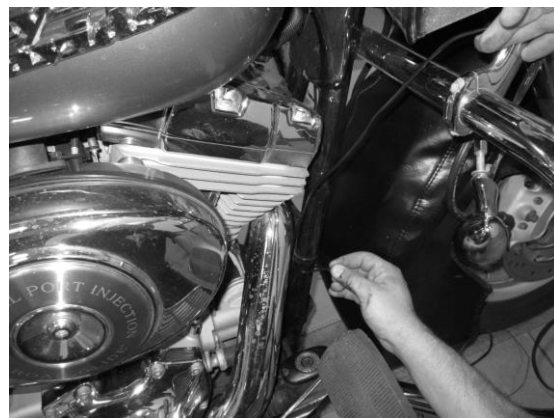
Tighten temp sensor with a 3/4" wrench
