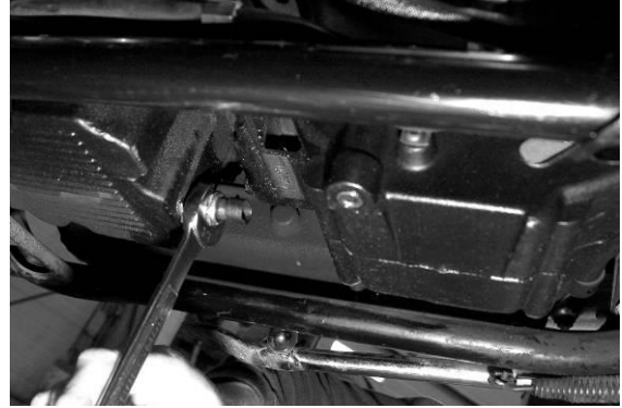
Tighten temp sensor with a 3/4" wrench
