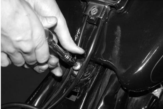
**Remove rear tank bolt**
