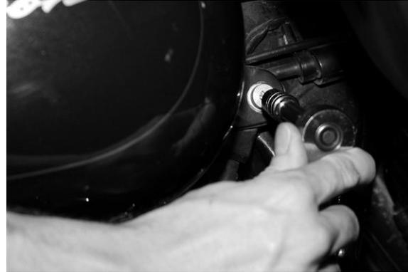
**Remove front tank bolts to loosen tank**
