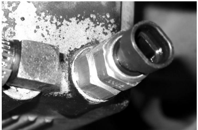
Temp sensor installed as drain plug EVO
