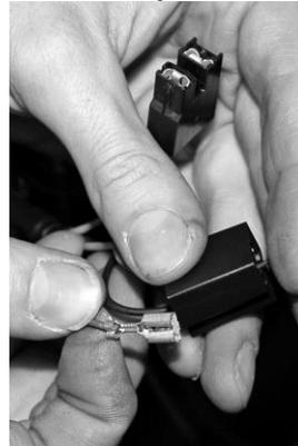
Remove the pin from the connector
