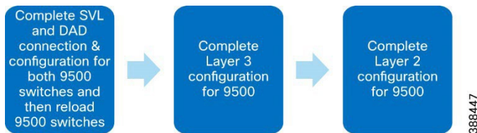
Figure 3-2: Workflow for Initial Bring-Up of Catalyst 9500 Series Switches in the Wind Farm OSS Core
