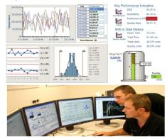
Supervisory Control And Data Acquisition System (SCADA) generally refers to an industrial control system performing a Centralized Alarm Management, Data Trending, and operator Display and Control of a process.
