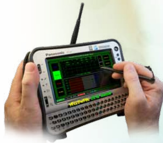
Berkeley Varitronics Systems' Tortoise Dual Band Transmitter (above) and YellowFin LTE Analyzer (below) are both used worldwide for the build out and optimization of 4G LTE networks.
