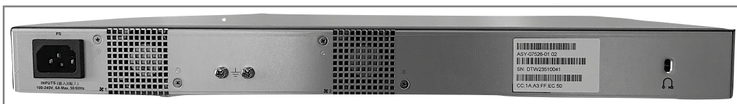
AWE-7220RP Rear (front to rear airflow)
