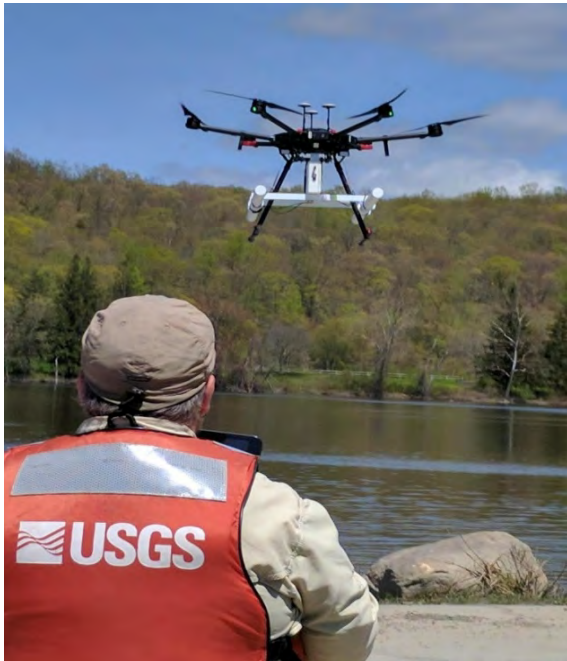
A USGS employee tests drone-based ground-penetrating radar. Source: USGS.
