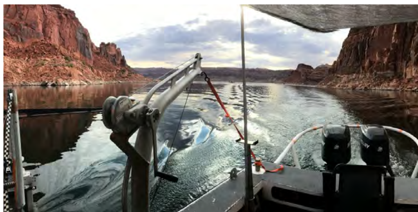
USGS Research Vessel Stephens operating within Lake Powell, Utah-Ariz. A multibeam echosounder is deployed off the starboard side of the vessel and is used to collect depth information within the reservoir. Source: USGS.
