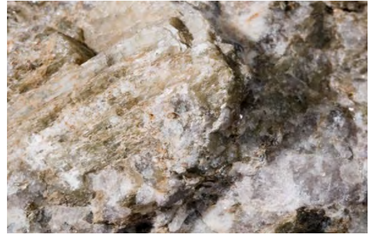
Spodumene, a primary mineral commodity of lithium. Uses include batteries for cell phones, laptops, and electric and hybrid vehicles. Source: USGS.
