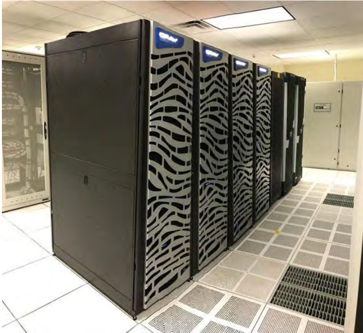
Advanced Research Computing (ARC)'s "Yeti" supercomputing cluster contains over 38,600 total cores; 23,800 GB of RAM; and 793 TB of usable storage. Source: USGS.
