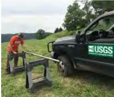
An acoustic televiewer for borehole geophysical logging in Monroe County, WV. Source: USGS.
