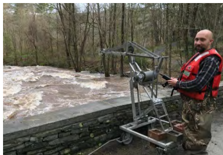
Left: USGS hydrographer Dave Thompson makes a near-peak flood measurement off a bridge at Tenmile River (Tusten, N.Y.). Right: USGS hydrographer Brent Hanson wades out in freezing waters to collect flood measurements on the Sheyenne River (Cooperstown, N. Dak). Source: USGS.
