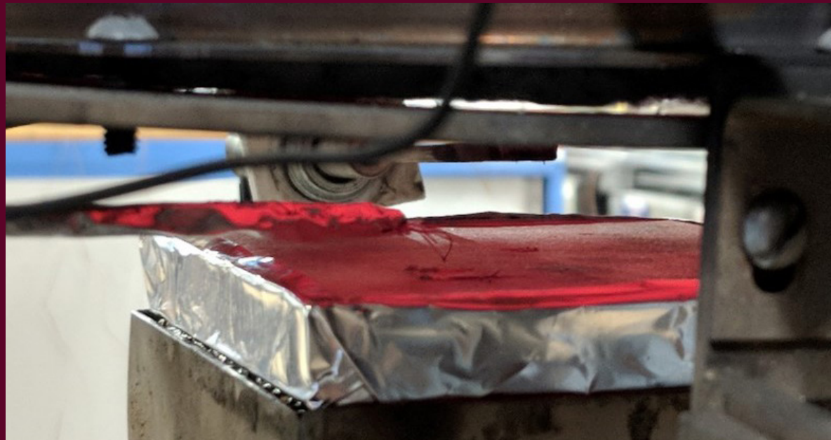
Figure 4: Cone calorimeter sample setup with surface temperature thermocouple measurement
