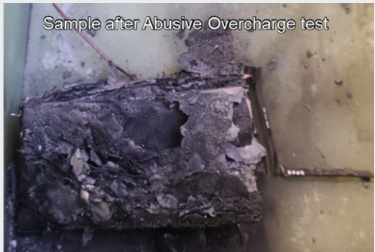
Figure 3 Battery samples after External Short-Circuit and Abusive Overcharge tests
