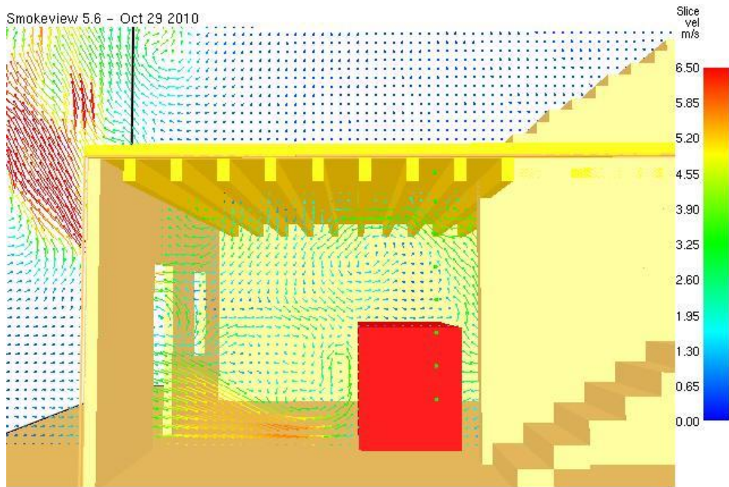
Figure 38 Velocity contours at a plane intersecting the middle of the basement door
