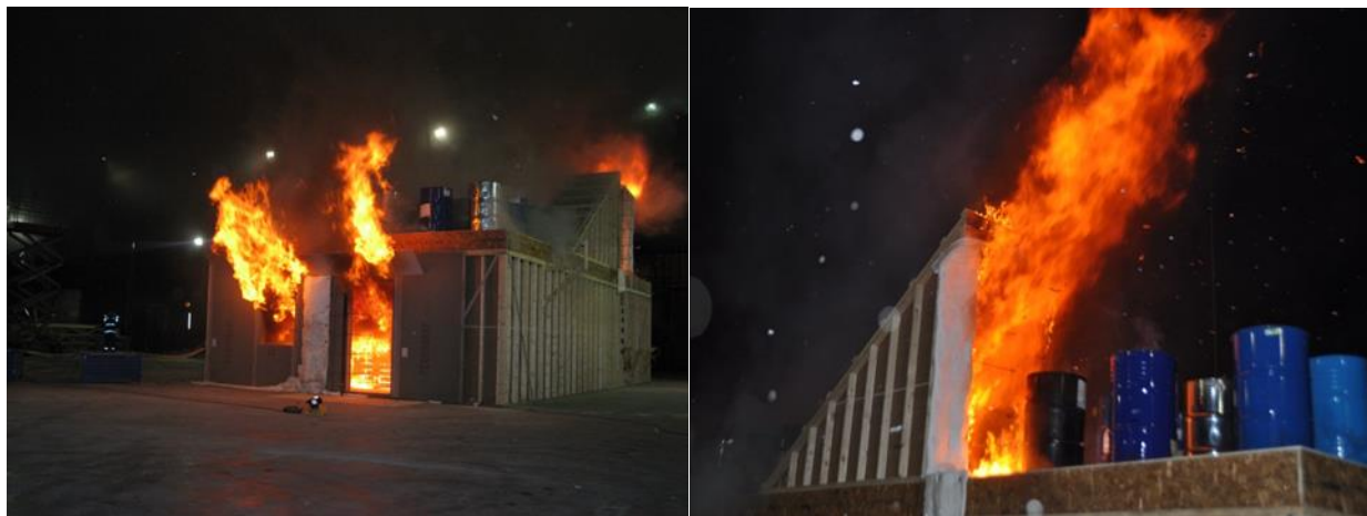
Figure 15 Pictures of flames through openings: front (left) stairway door at top (right)
