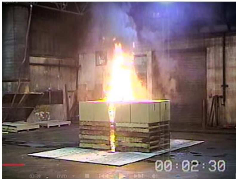
Figure 13 Photo of burning box/pallet stacks after 150s
