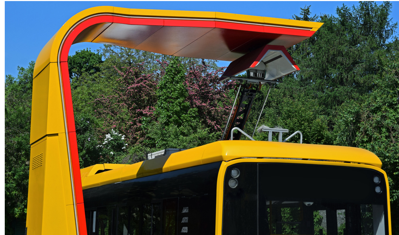
Figure 13 – Automatic Connection Means
