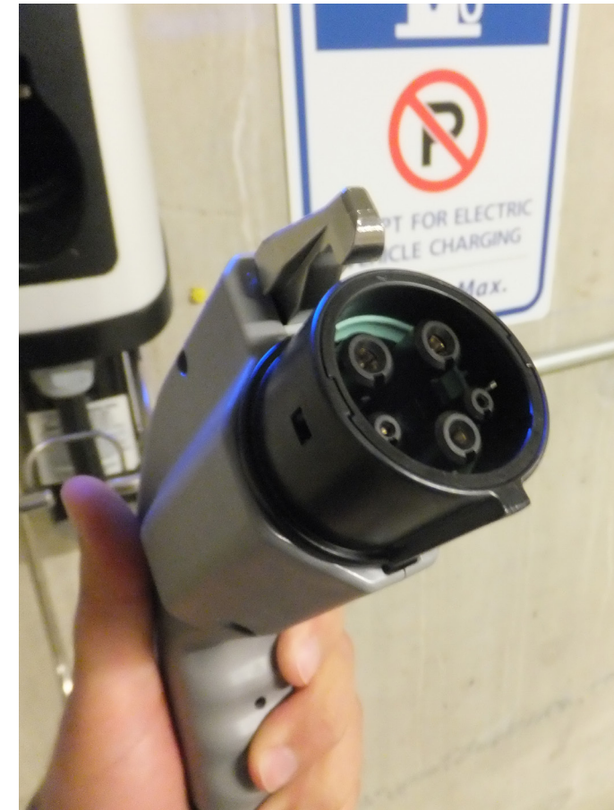
Figure 3 – SAE J1772 / Type 1 Configuration
