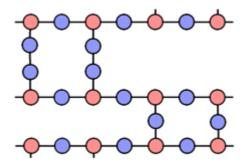
The bonds in polymers are mostly covalent. As a result, polymers have low thermal and electrical conductivities.
