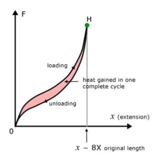
The graph illustrates how for a given force, the extension is greater for unloading than loading.
