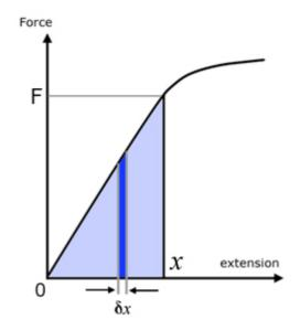
As can be seen from the graph, the area under the curve is half the product of F and X.
