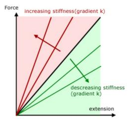
On a stress-strain graph the Young's Modulus is constant for the portion of the graph where Hooke's Law applies. This can be easily shown by substituting for k=F/x into the equation for E.
