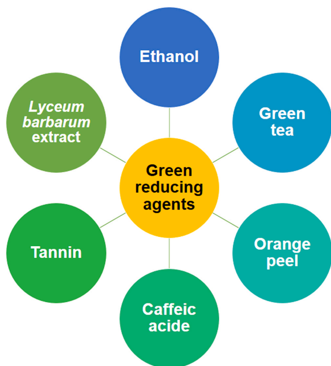
Fig. 5. Schematic diagram of the main types of green reducing agents for the synthesis of rGO.
