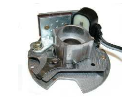
A single-pole reluctor system
