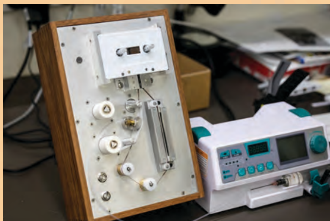
Audiocassette tape lubrication and cleaning machine designed and manufactured by AIATSIS engineering staff
