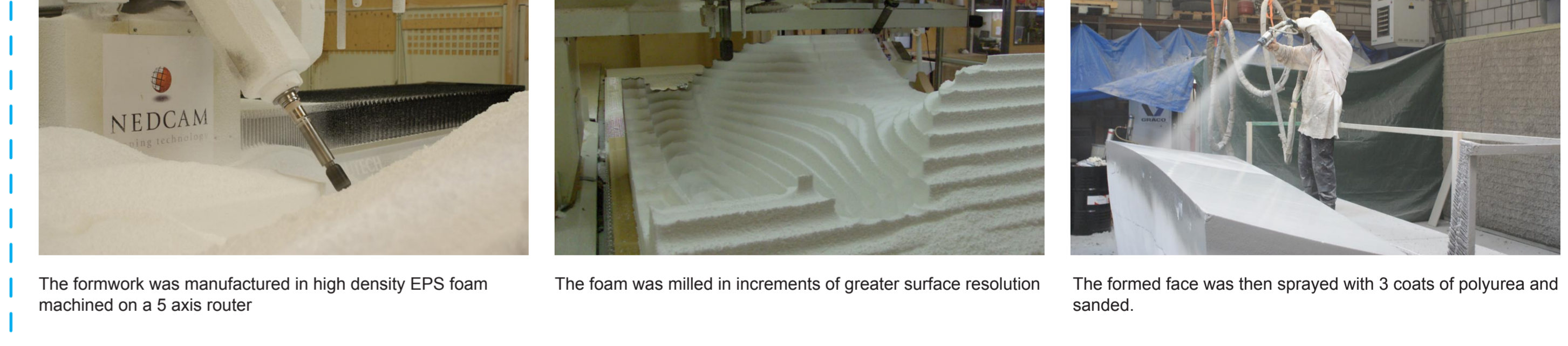
The geometry was remodelled in Solidworks to generate EPS moulds and control assembly tolerance.
